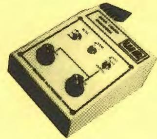
Using any source of composite video (colour or monochrome) and the Watford Beeb Video Digitiser, you can convert an image from your camera into a graphics screen on the BBC Micro.
