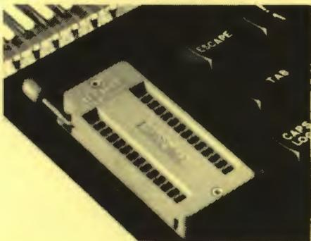
Allows you to change your ROMs quickly and efficiently, without opening the lid. The ZERO INSERTION FORCE (ZIF) socket is located into the ROM Cartridge's position.
