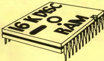
This is the RAM you've been waiting for!! This battery backed up, write protectable 16K sideways RAM board allows you to run from disk every sideways ROM available. Beware of other sideways RAM boards which are not backed up as certain ROMs will not run in these boards even though the RAM can be write protected. The Battery Backup facility allows retention of DATA after power off. On switch on the Micro will think the WATFORD DISC RAM is a ROM. Features available are:
